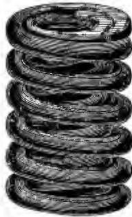
Fig. 5249. ROUND BAR DOUBLE-COIL SPIRAL-SPRING OR NEST-SPRING.
